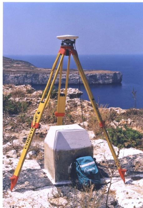
Fig.23 Receptor del GPS
