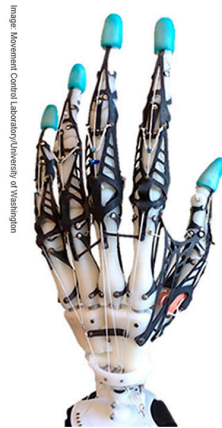
Figura 1.5: The University of Washington Hand [7].
