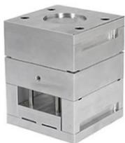
PCS Standard Aluminum Mold Bases are precision machined from 7075 aluminum. 23 standard frame size and plate thickness combinations are available. Aluminum mold bases have faster cycle times when compared to pre-hardened P-20 molds. Machining costs and lead-time is dramatically reduced when using an Aluminum Mold Base. Aluminum Mold Bases are made to order, please call PCS for lead time.
