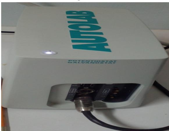
Figura 48: Potenciostato Autolab PGSTAT204
