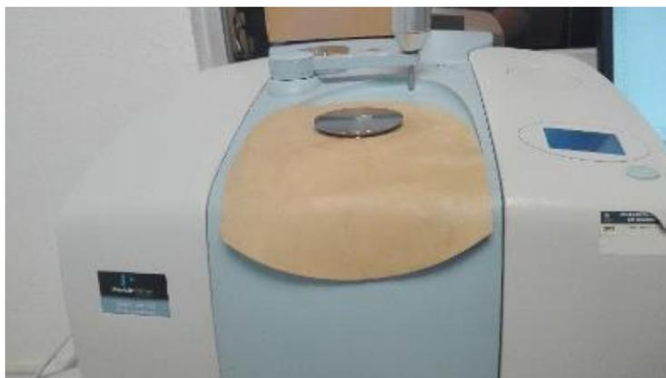
Figura 3.25 Espectrómetro FT-IR Spectrum 100 PerkinElmer Precisely.
